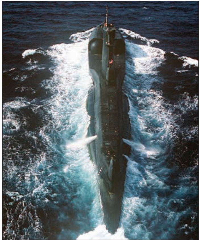
High-angle stern view of the USS Grayback underway. You can see two of the “sharkfin” sonar domes associated with the PUFFS system on the hull. (National Archives photo.)
