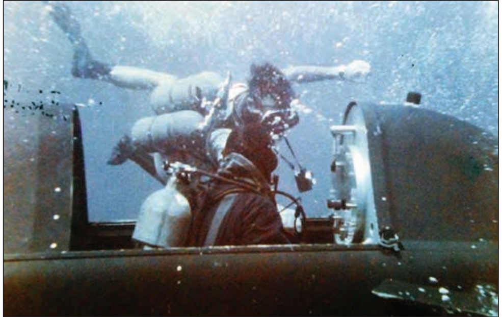
Divers from Grayback ready an SDV for launch operations at a depth of 35 feet. The vehicle was manned by personnel from Underwater Demolition Team 12. (National Archives photo.)
